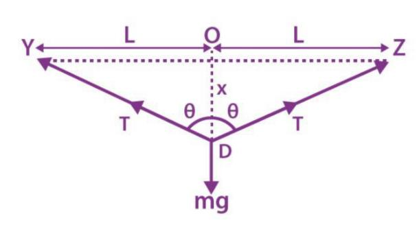
Let YZ be the mild steel wire of length 2I = 2m and cross sectional area  $A = 0.60 \times 10^{-2} \text{ cm}^2$ . Let the mass of m = 100 g = 0.1 kg be hung from the midpoint O, as shown in the figure. And let x be the depression at the midpoint i.e OD
