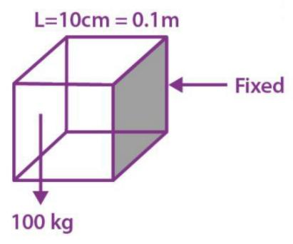
Edge of the aluminium cube, L = 10 cm =10/100= 0.1 m Area of each face,  $A = (0.1)^2 = 0.01$  m<sup>2</sup>
