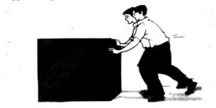
**Answer.** They can put rollers below the heavy load. Since, the rolling friction is smaller than the sliding friction. Therefore, putting rollers below the heavy load will make this task easier for them because rolling reduces friction.
