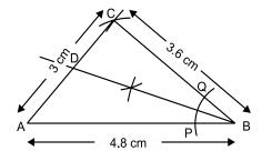
center 'B' draw an arc that intersect our line AB at P and line BC at Q. Step 5: With same radius and centre 'P' and 'Q' draw arcs which intersect at 'R'.
