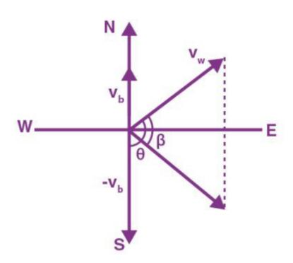
The angle between  $v_w$  and  $(-v_b)$  =  $90^\circ+~45^\circ$   $aneta=~{51\sin(90+45)\over72+51\cos(90+45)}$
