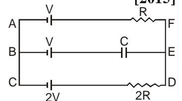
22. Find the charge on the capacitor as shown in the circuit. [2014]
