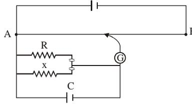
87. Figure, shows a 2.0 V potentiometer used for the determination of internal resistance of a 1.5 V cell. The balance point of the cell in open circuit is 76.3 cm. When a resistor of  $9.5 \Omega$  is used in the external circuit of the cell, the balance point shifts to 64.8 cm length of the potentiometer wire. Determine the internal resistance of the cell.
