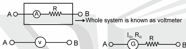
For maximum potential difference  $V = I_G \cdot R_s + I_G R_G$   $R_s = \frac{V}{I_G} - R_G$ . If  $R_G \ll R_s \Rightarrow R_s \approx \frac{V}{I_G}$
