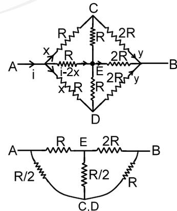
3. Find the equivalent Resistance between A and B
