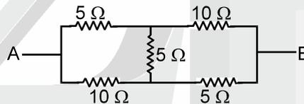
Sol. It is wheat stone bridge but not balanced. No series parallel connections. But similar values on input side and output. Here we see that even after using symmetry the circuit does not reduce to series parallel combination as in previous examples.
