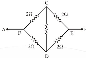
Calculate : (i) equivalent resistance of the network across the points A and B, and (ii) the magnitudes of currents flowing in the arms AFCEB and AFDEB.
