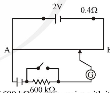
To ensure very low currents drawn from the standard cell, a very high resistance of  $600\text{ k}\Omega$  is put in series with it, which is shorted close to the balance point. The standard cell is then replaced by a cell of unknown emf  $\epsilon$  and the balance point found similarly, turns out to be at 82.3 cm length of the wire.
