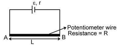
Potential gradient ( $x$ )  $\rightarrow$  Potential difference per unit length of wire  $x = \frac{V_A - V_B}{L} = \frac{\epsilon}{R+r} \cdot \frac{R}{L}$
