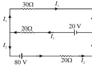
33. In the given circuit, assuming point A to be at zero potential, use Kirchhoff's rules to determine the potential at point B. [All India 2011]
