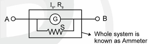
If maximum value of current to be measured by ammeter is  $I$  then  $I_g \cdot R_g = (I - I_g)S$
