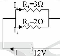
(a) equivalent resistance of the parallel combination, (b) the circuit current and (c) the branch currents.
