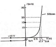
The V-I characteristic of a diode is shown in the figure. The ratio of the resistance of the diode at I = 15 mA to the resistance at V = -10 V is
